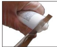
Cut end of cartridge off to open
