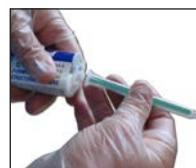
For 50ml dual cartridge, use nozzle and gun to dispense
