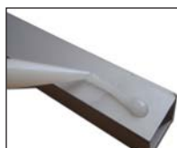
Apply adhesive as a continuous bead
