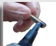
Apply adhesive, take care not to contaminate nozzle
