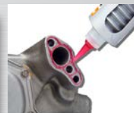
Apply adhesive as a continuous bead, encircle bolt holes
