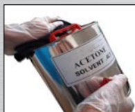
Abrade & degrease with solvent
