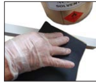
Abrade with wet and dry grit paper
