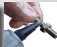
Adhesive should be applied where there is maximum contact
