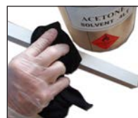
Degrease with solvent
