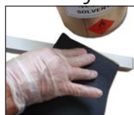
Abrade with wet and dry grit paper
